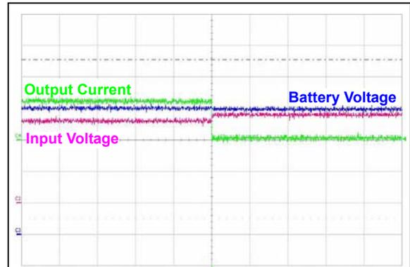
**FIGURE 2-16:** Complete Charge Cycle (875 mAh Li-Ion Battery).
