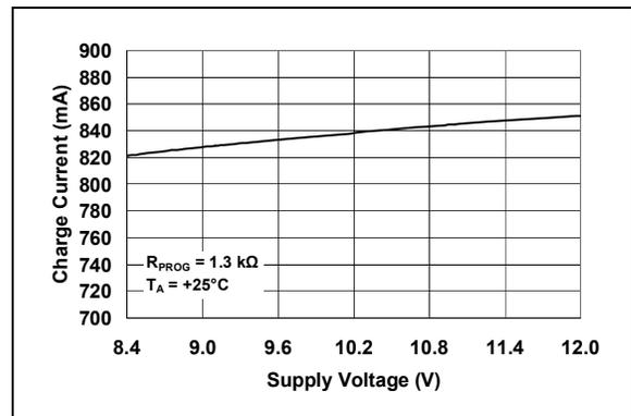
**FIGURE 2-6:** Charge Current ( $I_{OUT}$ ) vs. Supply Voltage ( $V_{DD}$ ).
