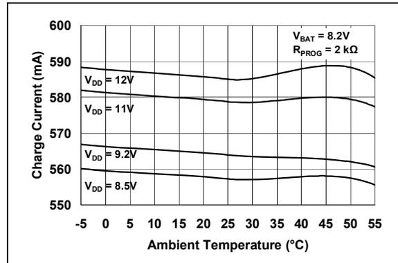
**FIGURE 2-10:** Charge Current ( $I_{OUT}$ ) vs. Ambient Temperature ( $T_A$ ).
